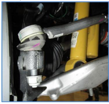
6. Disconnect the sway bar links on both sides of the vehicle. Remove the nut using a 21mm wrench, you may need to hold the stud with a hex key to keep the stud from spinning.
