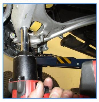
4. Separate the upper control arm from the knuckle. Using an 18mm wrench or socket remove the nut for the control arm ball joint, then disconnect upper arm from knuckle.
