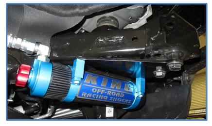
19. Install the 1/4 X 1" bolts (CB1501) in the reservoir clamps and tighten using a 3/16 Allen wrench.
