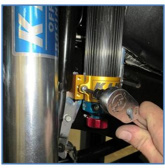
11. Place the rod end into the lower mount, install the factory bolt and tighten to factory specs.
