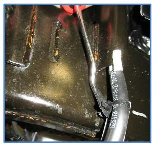
5. <u>Installing reservoir brackets</u> – First attach the clamp to the reservoir bracket with the provided 1/4 X 1" FHCS (CB5501) using a 5/32 Allen wrench. Be aware the brackets are side specific. Photos show the RIGHT SIDE. See below for proper orientation.
