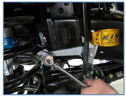
9. <u>Installing Shocks</u> – Be aware the shocks are side specific, make sure you have the proper shock for the side you are working on (photos below show LEFT SIDE). Begin placing the shock into position on the vehicle while inserting the reservoir into the clamp. Place the end cap into the upper mount, install the factory bolt and tighten to factory specs.
