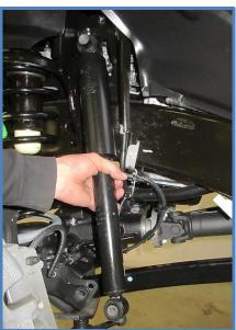
3. Remove the brake line bracket bolt using a 10mm wrench or socket.
