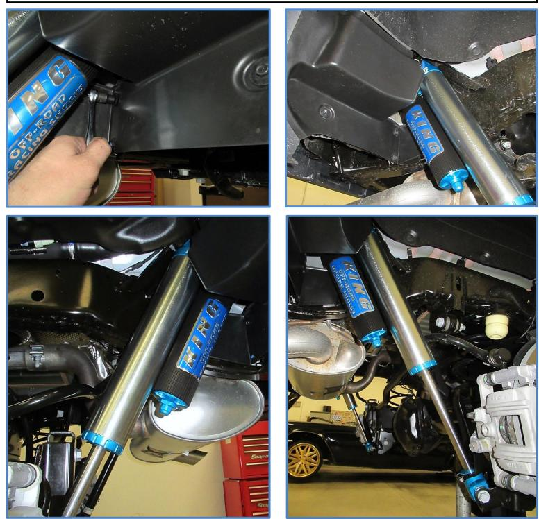
**DOUBLE CHECK ALL HARDWARE:** Make sure everything is installed correctly and all hardware is tight before reinstalling tires. Install tires; remove jack stands and lower vehicle to the ground. Recheck all hardware and lug nuts after 100 miles and periodically after that as part of routine maintenance.
