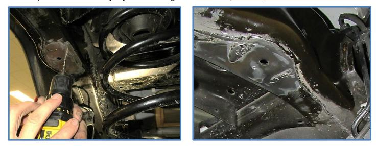
7. Drill the large hole using a 2-5/16" hole saw. Line up the center pilot bit of hole saw with the new pilot hole you just drilled and drill through the bottom of the frame.
