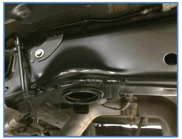
13. Reinstall the brake line brackets to the frame.
