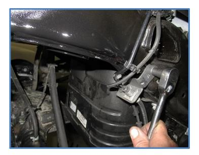
14. <u>Install bump stops and adjust position</u> – You will need to install bump stops and adjust the position before you finalize installation. If you are using the 1.5" stroke bump stops then you will most likely thread them all the way in as shown below. The 1.5" stroke bump stops are intended for maximizing up travel on stock vehicles with no lift or with mild lifts up to 2".
