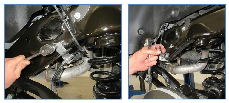
3. Using a cut off wheel or reciprocating saw cut the small welds on each side of the factory foam bump stop mount. Carefully cut the welds only, do not cut into the frame!
