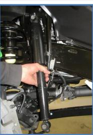
3. Install King Shocks using the factory hardware. Place the shock in the upper mount with the longer spacer facing in towards the frame. Insert the factory bolt and tighten to factory specs. Install shocks with cylinder on top and shaft mounted to the axle as shown.
