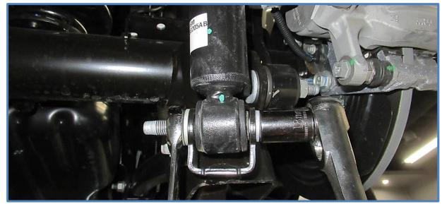
3. Remove upper bolt using an 18mm wrench or socket and remove shock.
