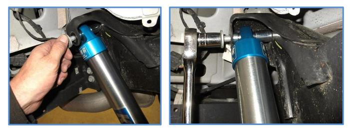
5. Place the rod end in the lower mount and install the factory bolt and nut. Tighten to factory specs.
