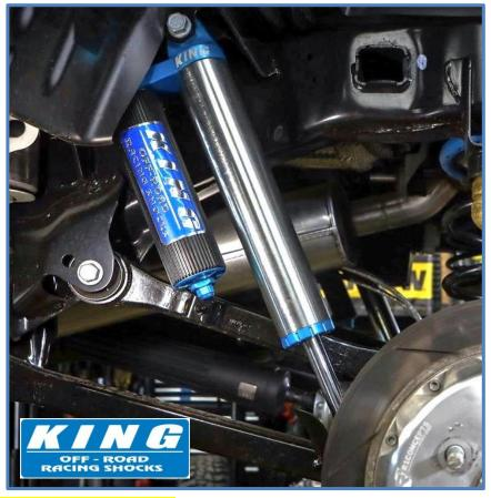
**DOUBLE CHECK ALL HARDWARE:** Make sure everything is installed correctly and all hardware is tight before reinstalling tires. Install tires, remove jack stands and lower vehicle to the ground. Recheck all hardware and lug nuts after 100 miles and periodically after that as part of routine maintenance.
