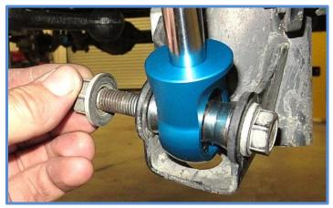
**DOUBLE CHECK ALL HARDWARE:** Make sure everything is installed correctly and all hardware is tight. Remove jack stands and lower vehicle to the ground. Recheck all hardware and lug nuts after 100 miles and periodically after that as part of routine maintenance.
