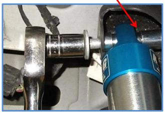
4. Place the rod end in the lower mount, install the factory hardware and tighten to factory specs.
