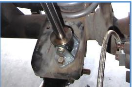
2. Be aware that the shocks are side specific and must be mounted so that the reservoir is next to the spring. Remove the nut, washer, retaining washer and upper bushing from the shock. Install shocks by inserting the mounting pin into the upper mount on vehicle with the thick bushing on bottom, then place the thinner bushing, retaining washer and regular washer on top and thread the nut onto the stud finger tight for now.
