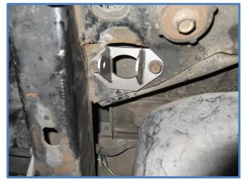
2. Install King Shocks... Shock mounting for the rear on Jeep TJ's can vary from one vehicle to the next depending on factory options and aftermarket lift kits and accessories. Begin by installing shocks as labeled Left and Right. Place the end cap up into the bar pin eliminator bracket and install the 3/8" hardware provided with the shock. Place the rod end in the lower mount and install the factory bolt. Tighten upper 3/8" bolt to 35 ft/lbs. Tighten lower bolt to factory specs.
