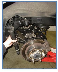
3. Slide the provided spacer onto the lower mounting stud, then place the rod end on the stud followed by the other bearing spacer. Install the factory bolt and tighten to factory specs.
