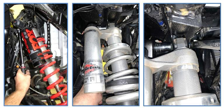
4. Install King Shocks using the factory hardware. Be aware the shocks are side specific. Place the shock in the upper mount with the reservoir towards the rear of the vehicle and install the factory bolt and nut.
