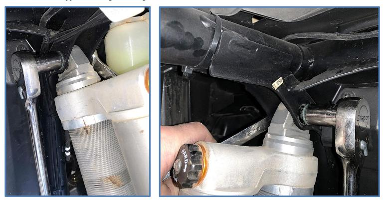
4. Install King Shocks using the factory hardware. Be aware the shocks are side specific. Place the shock in the upper mount with the reservoir facing out towards the tire and back towards the rear of the vehicle. Install the factory bolt and nut in the upper mount.
