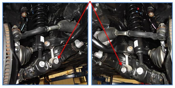
2. Disconnect the tie rod end by first removing pin using needle nose pliers, then remove nut using a 24mm socket and separate tie rod from steering knuckle.
