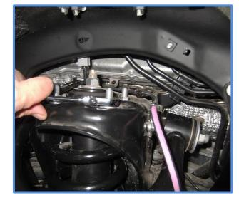
9. Once the factory shock has been taken off the vehicle, unbolt and remove the factory upper control arm by removing the long through bolt located behind the coil bucket. Install the King Coilover with the control arms removed then install aftermarket arms as per the instructions that came with your control arms.
