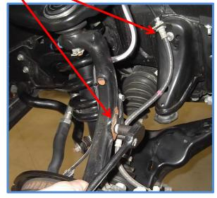
6. Remove upper ball joint nut using a 19mm socket. Separate upper A-arm from spindle.
