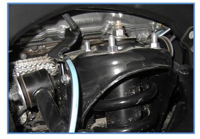
8. Remove the lower mounting bolt using a 22mm wrench and socket. Remove factory shock.
