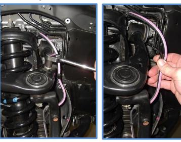
5. Pull the pin out of the ball joint stud in the upper control arm using needle nose pliers.
