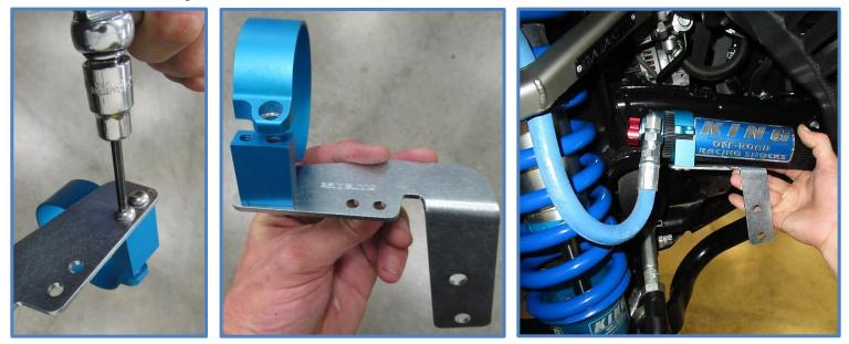
16. Bolt reservoir bracket to frame using the factory bolts and plastic piece as shown below. Once the bracket is secure, adjust reservoir as needed and tighten clamps using the 1/4 x 1" SHCS (CB1501).
