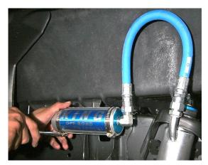
(4) Install your King Shocks using the factory hardware for the lower mount and the supplied hardware for the upper mount. Make sure that you have a rubber bushing on each side of the upper shock mount. Attach the remote reservoir to the mount using the supplied band clamps as shown.
