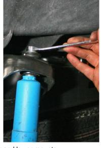
(3) Remove the factory shocks by removing the hardware from the upper and lower mounts.
