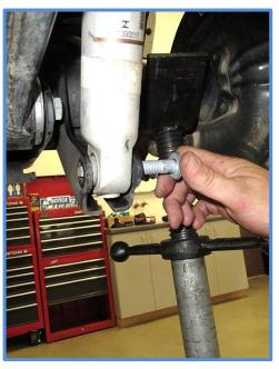
3. Remove the nut from the upper mount using an 18mm wrench or socket and remove shock from vehicle.
