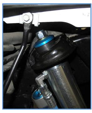
Important Note: The rubber bushings on your King shocks are different from each other. Make sure the taller bushing is on the bottom next to the body of the shock as shown. The silver washer between the rubber bushings represents the material thickness of the upper shock mount. It's important to tighten the nut only until the rubber bushings start to compress. There should be approximately 1/8" – 3/16" of the mounting pin protruding above the nut.
