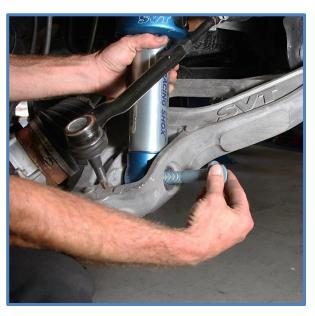
8. Remove the factory shock from the vehicle as shown.
