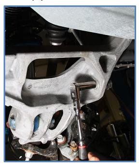
15. Reinstall the brake/ABS line brackets.
