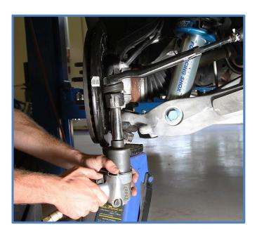
4. Remove the sway bar bolts from the lower a-arm.
