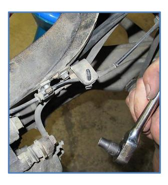
16. Install reservoir brackets to the bottom of the frame using the skid plate bolt and bracket. Unbolt the skid plate and bracket and install reservoir brackets as shown below.
