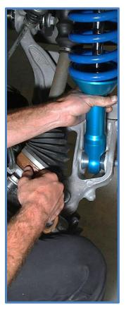
10. Place the HD 3/8" washers (CW1701) on the upper mounting studs followed by the 3/8" Nylock nuts (CN2711). Tighten nuts to 35ft-lbs.
