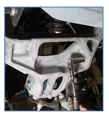
5. Loosen the lower shock bolt but do not remove.
