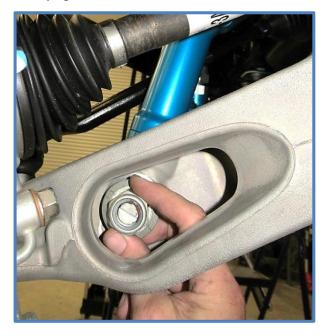
12. Reconnect upper control arms to spindle and tighten to factory specs.
