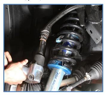
3. Disconnect tie rod ends from steering knuckle.
