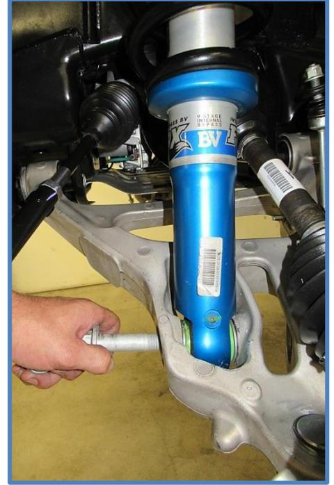
5. Remove the upper ball joint nut using an 18mm socket. Separate the upper control arm from the spindle.
