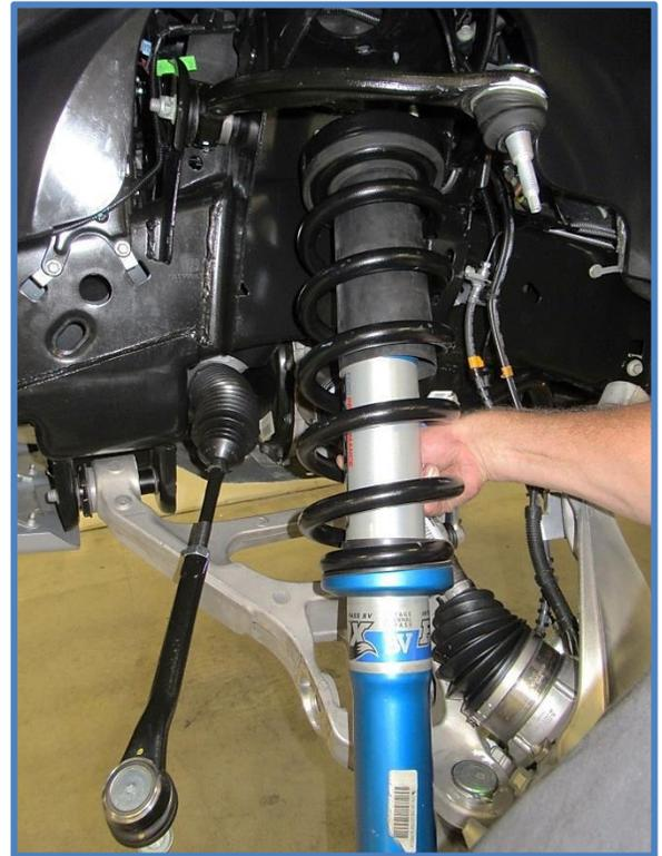
8. **Install King Shocks** – Place the coilover in position on the vehicle by inserting the upper mount with mounting studs into the upper mount (coil bucket) on the vehicle. Then, while pushing down on lower control arm, get the rod end into the mounting pocket on the lower control arm. Be aware the shocks are side specific and can only be mounted on the designated side. Photos below show the left side.
