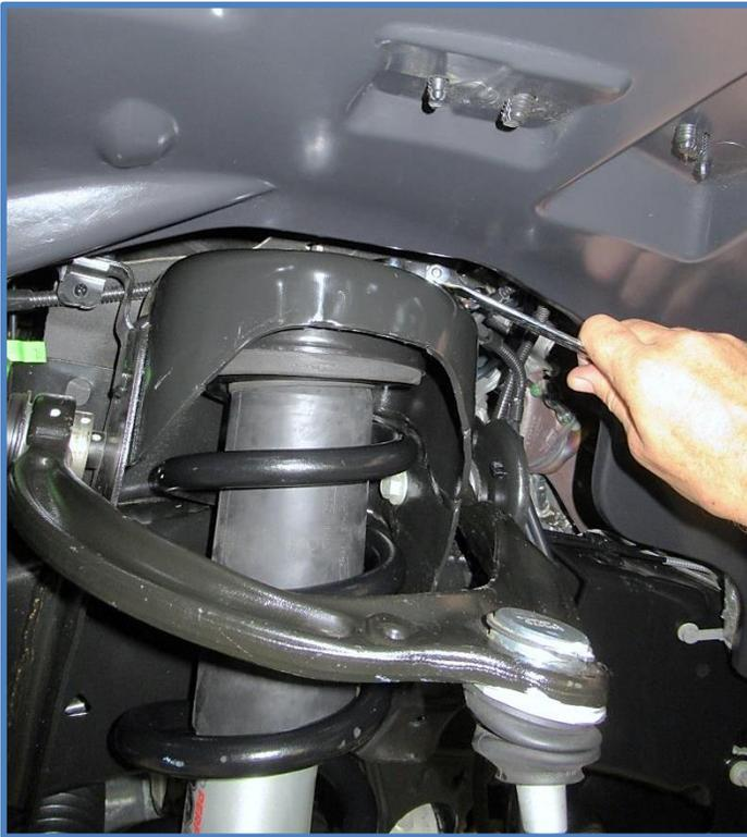
7. Remove factory shocks. You will need to push down on lower control arm to remove shock.
