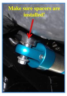
4. Place the rod end with tapered spacer into the drag link and install the provided 10mm x 80mm bolt with washer. Then install washer and nut on bolt and tighten with a 17mm wrench and socket.
