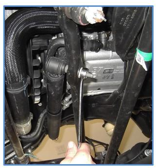
2. Remove bolt from frame end using a 15mm wrench or socket and remove stabilizer.
