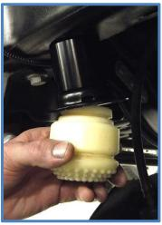
8. Remove the lower coil mount using an 18mm Socket.
