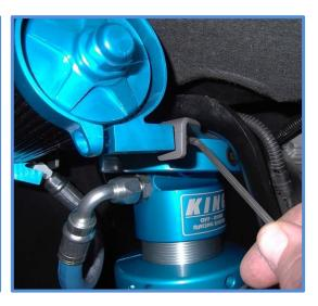
20. Center reservoir in the bracket and insert the provided 1" socket head cap screws in the clamps and tighten with a 3/16 allen wrench to secure reservoir. Hose should be pointing back as shown below.
