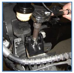
10. Using the reservoir bracket as a template carefully mark the holes in the upper coil spring mount. Mark holes, then center punch each hole and recheck the alignment of marked holes with reservoir bracket.
