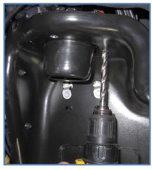
12. Cut the coil spring locating boss flush with the upper mount. Grind any protruding or sharp edges so the surface is completely flat. Paint the bare metal prior to installing shocks to prevent rusting.
