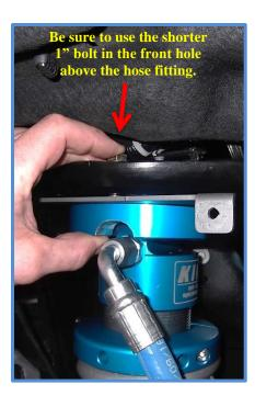
16. Install upper mounting bolts and tighten to 35 ft.lbs. using a 9/16 wrench/socket.
