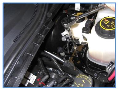
18. For 2.5 kits with standard reservoir, place the reservoir in the reservoir bracket and install the provided hose clamps. Center the reservoir in the cradle and twist the reservoir towards you to twist the hose in towards the wheel well and tighten the clamps.
