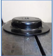
7. Reinstall the bump stop mount with the supplied spacer and longer bolt w/washer. Tighten the bolt using a 6mm Allen wrench. Push the bump stop back into the mount making sure it's pushed in all the way.
