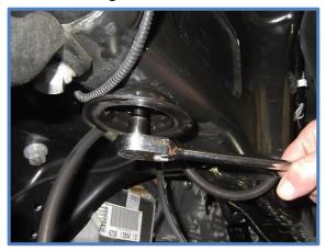
6. The bump stop mount has a tab sticking out that needs to be tapped flat with a hammer as shown.
