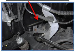
3. With the shocks removed and the ABS/brake lines disconnected, lower the axle and remove the coil springs.
