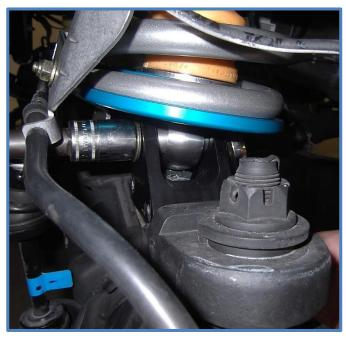
14. On the left side of some vehicles you will need to move the brake proportioning unit to install the upper mounting bolts. First remove the bolt on the front side of the coil mount using a 13mm wrench/socket. Then find the two nuts located inside the engine compartment and just loosen those nuts to the end of the stud but do not remove. This should give you room to pry the brake unit up enough to install bolts.
