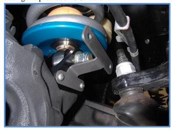
22. Attach the brake line to the previously installed brake line support by placing the tab in the inward hole and install the ¼ x ¾ bolt with washer in the outward hole making sure the head of bolt is on the same side as shock. Install washer and nut and tighten with 7/16 wrench and socket.
