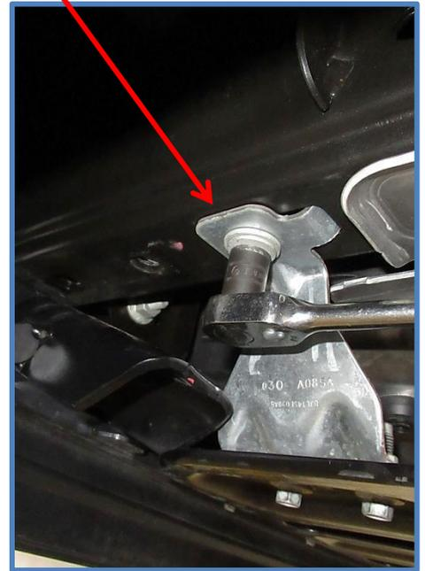
Place the reservoir mount against frame between the frame and tow hook (and skid plate if applicable). Install the two tow hook factory bolts you just removed. If you have the skid plate option you will need to place one of the thick washers from the hardware kit (CW1701) between the frame and skid plate, install factory bolt and tighten. Tighten all bolts to factory specs. Reservoir brackets are side specific, see photos for proper mounting.
