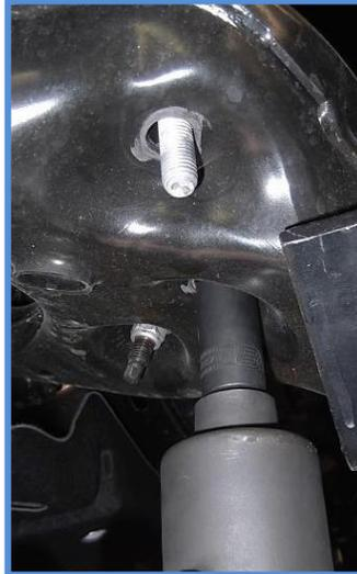
6. Using an 18mm wrench/socket, remove the three nuts from the top of the shock assembly.
