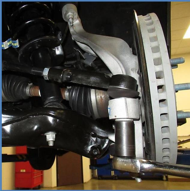
3. Disconnect the upper A-arm from the upright. Using a 18mm wrench/socket, loosen the nut on the ball joint. Separate the ball joint from the upright using proper ball joint tools. You may need to use an 8mm wrench to hold the stud as shown below.
