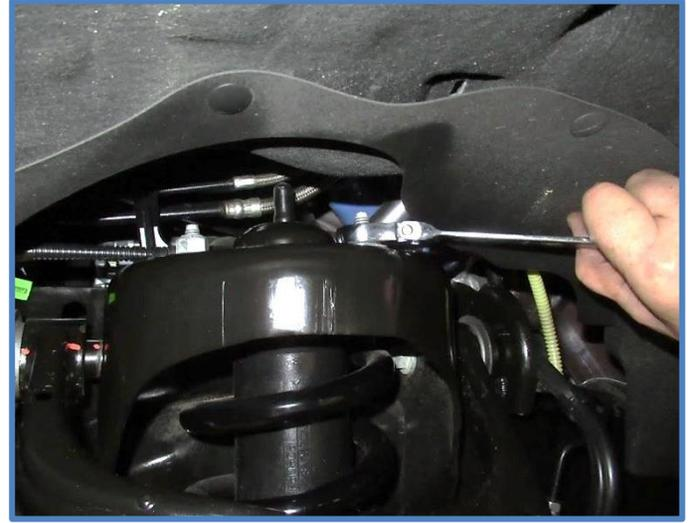
7. Remove shocks from vehicle by pushing down on lower control arm while holding the shock up, pull the studs out of the lower mount and remove shock.
