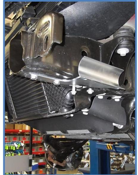
9. Install King Remote Reservoir Shocks by first feeding the reservoir through the hole at the top of the shock mount, then place the shock in position on the vehicle. Get the shocks in position on both sides of the vehicle before reconnecting any suspension components. Shocks are side specific, the reservoir will route towards the front of vehicle as shown below.
