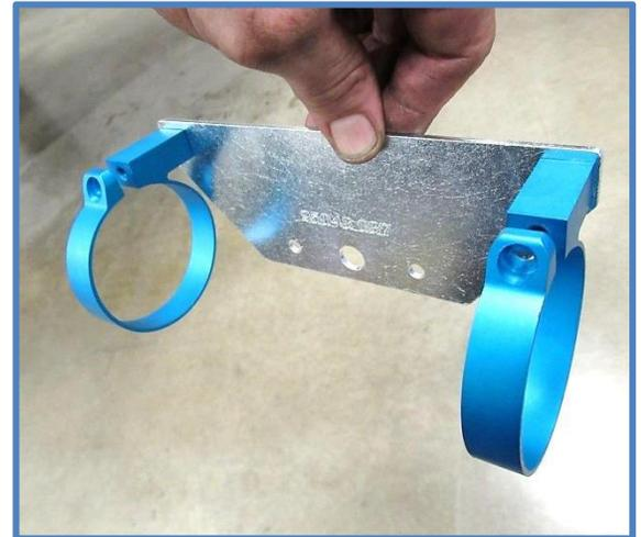
11. Attach reservoir brackets to the vehicle using the threaded nut plate and hardware from the kit. First thread the 1/4 X 2.5" SHCS into the center hole of the nut plate, this is just for holding the nut plate while attaching reservoir bracket.
