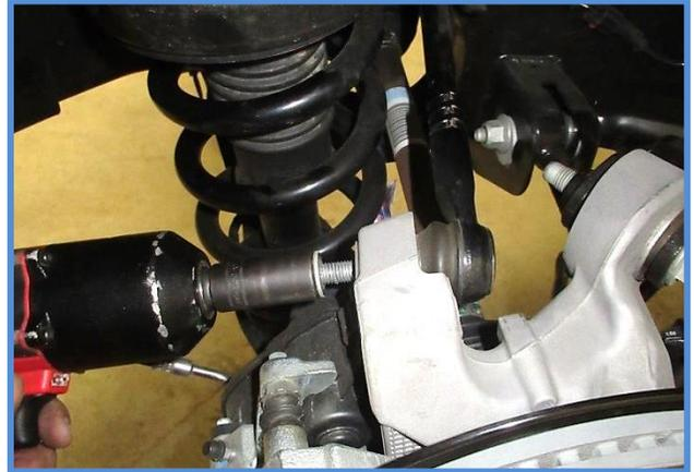
4. Remove the bolt from the other upper link using a 24mm socket (nut is welded).
