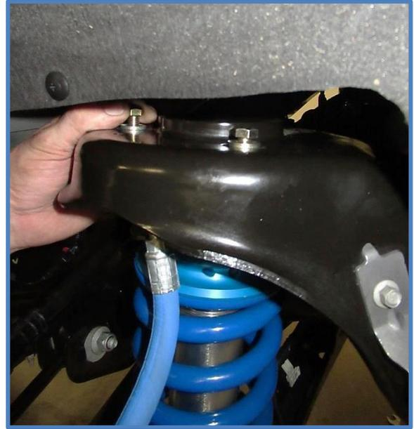
7. Place a jack under the lower control arm and raise the arm up until the shock mount in the lower control arm is in line with the shock. Install the factory bolt and tighten to factory specs. Now tighten the upper mounting bolts to 35 ft. lbs.
