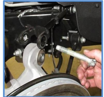
5. Remove the 3 nuts from the upper mount of the shock using a 15mm wrench/socket and remove the shock.
