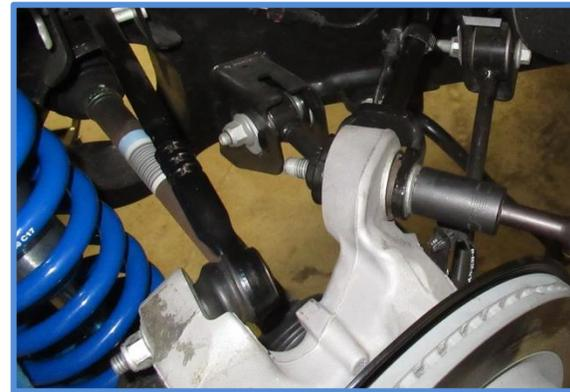
9. Reconnect the sway bar links and tighten to factory specs.
