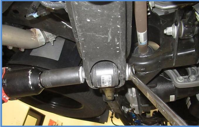
3. Remove the nut from the ball joint on the upper link using an 18mm socket. Separate ball joint from the knuckle.
