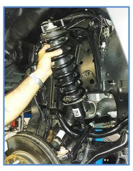
6. Install King Shocks. Be aware the shocks are side specific; make sure you are installing the shocks on the proper side. Start by placing the shock in position on the vehicle and install the factory lower mounting bolt.
