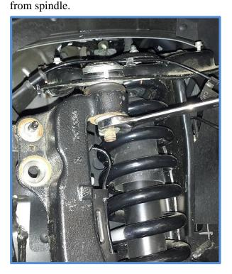
4. Remove the lower shock mount bolt.
