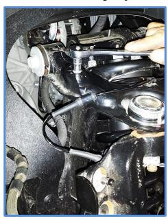
3. Remove cotter pin from upper A-arm ball joint stud then remove nut and separate upper A-arm 4. Remove the
