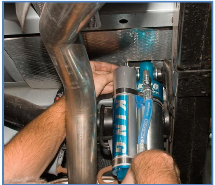
5. Place the rod end in the lower shock mount and install the factory bolt. Tighten lower mounting bolts to factory specs.
