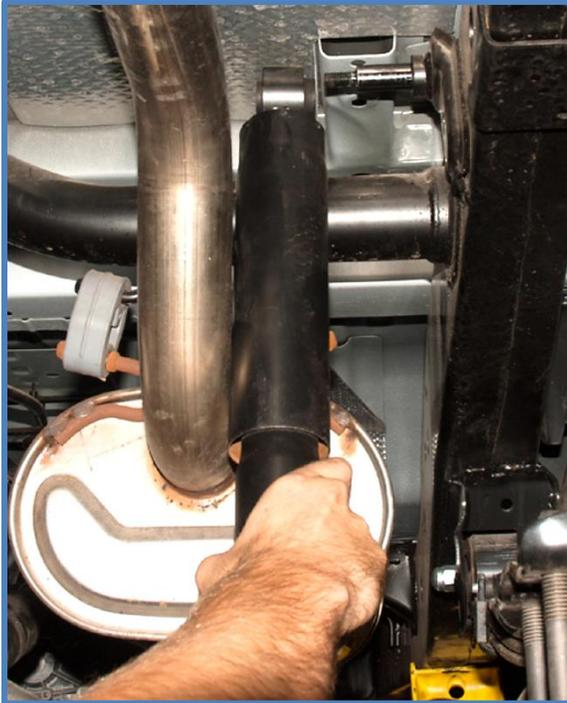
4. Install King Shocks. Shocks are side specific, make sure you are installing the shocks on the proper side. Place shock on upper mounting stud, install factory nut and tighten to factory specs.
