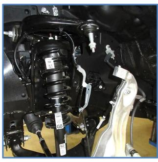
6. Complete steps 1-5 on both sides of the vehicle, then remove shocks. Remove shocks by pushing down on the lower control arm while pulling the top of shock out of the upper mount then lift the shock out of lower control arm and remove from vehicle.
