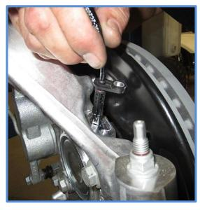
3. Remove the upper mounting nuts using a 15mm wrench or socket.
