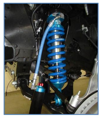
8. Install the provided 3/8" upper mounting bolts with HD washers (CW1701). Use the longer 3/8 X 1" bolts (CB4701) in the two holes on the back side of the upper mount. Use the shorter 3/8 X 3/4" bolt (CB4702) in the front hole above the hose fitting. Thread the bolts in to hold shock in place but do not tighten yet.
