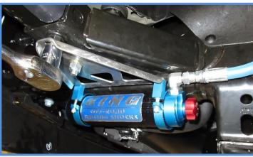
16. Install the 1/4 X 1" bolts (CB1501) in the reservoir clamps and tighten using a 3/16 Allen wrench.
