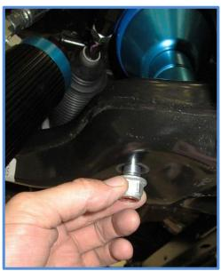
10. Reconnect the upper control arm and tighten nut to factory specs. You may need to hold the stud with an 8mm wrench as shown below to keep the ball joint from spinning while tightening nut.
