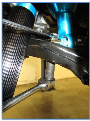
12. Install the ABS sensor, ABS bracket and brake line bracket.
