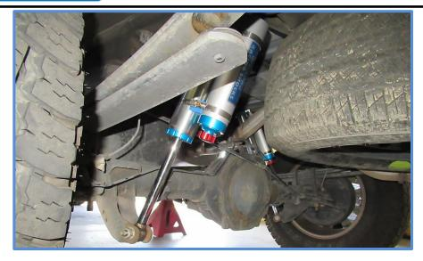
Some Chevy's and GMC's have clearance issues with our 2.5 piggyback rear shock, if shocks will not fit with reservoir end mounted to the frame then you can mount shocks with shaft up and reservoir end mounted to axle as shown.
