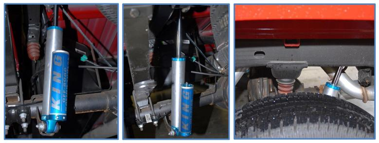
Make sure shocks are installed properly and all hardware is tight. Remove jack stands and lower vehicle. Double check all hardware after 100 miles or so and periodically after that as part of routine maintenance.
