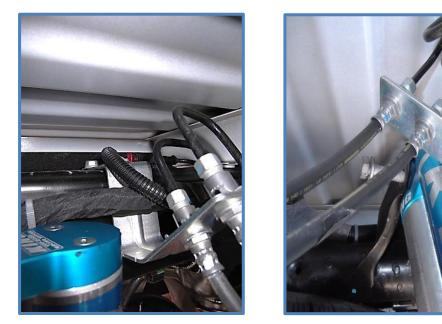
3. <u>For shocks with Compression Adjusters:</u> Shocks with compression adjusters need to be mounted so that the reservoirs are both facing towards the rear of the vehicle. Use factory hardware to install shocks and torque to factory specs.
