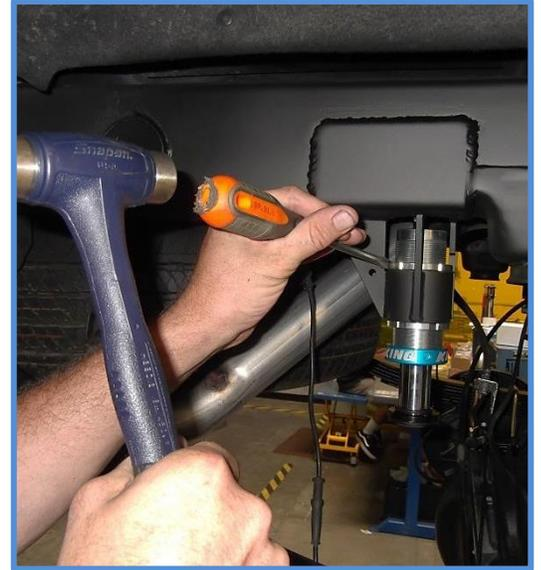
Tighten set screws when final position has been determined
