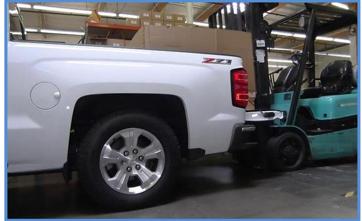
8. With the suspension bottomed out, check for clearance issues. On the left side make sure the bump stop has clearance between the bump stop and the strike pad. Also on the left side make sure the lower strike pad does not contact the gas tank. Make any necessary adjustments. On the right side make sure the bump stop has clearance between bump stop and the strike pad. Make any necessary adjustments at this time.
