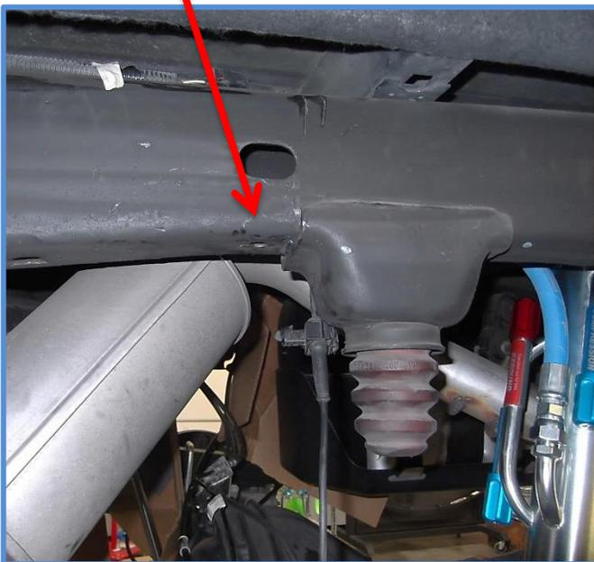
2. Remove factory bump stops using a 10mm socket to remove the bolt located inside the foam bump.
