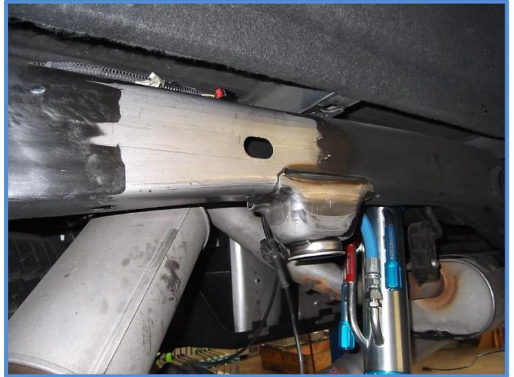
4. Next prepare your axle for welding. Grind the paint from the existing bump pad on the axle and the shock mount area as shown below.
