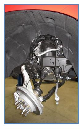
7. If you are installing aftermarket upper control arms, install those now while the shocks are removed. Use a 21mm wrench and socket to remove the factory bolts for the upper control arms. Install the aftermarket upper control arms per the instructions that came with your control arms.
