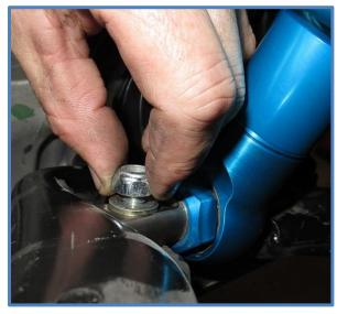
11. Reconnect upper control arm to knuckle and tighten hardware to factory specs. Connect aftermarket upper arms using the instructions provided with your control arms.
