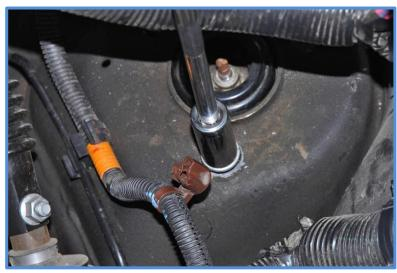
3. Using a 15mm socket, remove the lower shock mount bolts then remove the factory shock.
