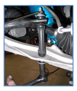
12. Pay special attention to brake lines, ABS lines etc. Make sure you have enough slack at full droop and full turn. Make sure there are no interference/clearance issues or lines that can get caught on moving parts.
