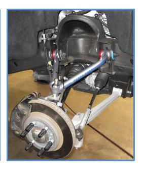
6. Install King Shocks. Shocks are side specific, be sure you are installing the shocks on the proper side. Place the shock in position on the vehicle and install the 10mm lower mounting bolts w/washers, nuts provided in the kit but do not tighten.
