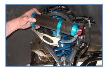
9. Place a jack under the lower control arm and jack the arm up until the upper mounting plate is tight against the coil bucket. Place the reservoir bracket over the studs and install the provided 3/8" washers and nuts and tighten. Now tighten the lower hardware, with all the hardware tight you can lower and remove the jack.
