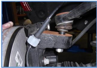
4. Using a 15mm socket, remove the lower shock mount bolts then remove the factory shock.
