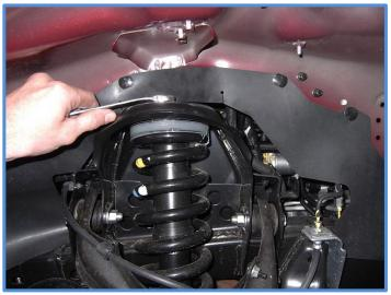
4. Line up the upper mounting plate on shock with the upper mount on the vehicle and place the reservoir bracket on top of the upper mount. Use the supplied 3/8" bolts and install through the reservoir bracket and upper mount and thread into the upper mounting plate on shock. Be sure to use the shorter 3/8 x 3/4" bolt in the front hole above the hose fitting and the longer 1" bolts in the back two holes, Failure to do
