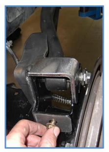
9. Place one of the ABS line clips back into the provided hole in the control arm bracket.
