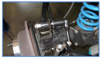
8. Slide the Strike Pad over the control arm bracket. Strike Pad may fit fairly tight and will need to be tapped into position with a mallet. Install the provided longer 14mm bolt and reuse the factory nut but do not tighten. Then install the provided 3/8 bolts with washers and nuts but do not tighten. With both bolts in place go ahead and tighten the control arm bolt first then tighten the 3/8 bolts.
