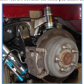
If the Strike Pad touches the bulge in frame then grind the bulge.
