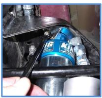
4. Put the rod end into the lower shock mount, insert the bolt, install nut and tighten.
