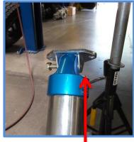
3. To make installation easier, remove the nut from the top mount as shown above. You can slide the bolt over to gain access to the factory mounting bolts above it. Insert the shock assembly into the frame pockets, Install the factory mounting bolts and tighten. After the mounting bolts are tightened install the nut and washer to the through bolt on shock and tighten.
