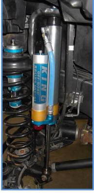
Important Note: The rubber bushings on your King Shocks are different from each other. Make sure the taller bushing is on the bottom next to the body of the shock as shown. The silver washer between the rubber bushings represents the material thickness of the upper shock mount. It's important to tighten the nut only until the rubber bushings start to compress. There should be approximately 1/8" – 3/16" of the mounting pin protruding above the nut.
