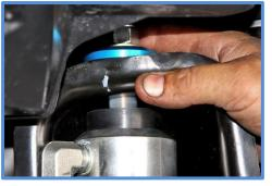
3. Install factory nut and bolt for lower mount and tighten. Jack up the axle so that the shock is tight against the upper mount and tighten nut so that the bushing just starts to compress, do not overtighten nuts.
