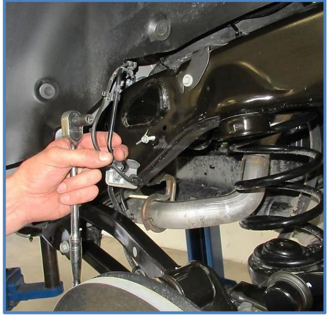
3. Using a cut off wheel or reciprocating saw cut the small welds on each side of the factory foam bump stop mount. Carefully cut the welds only, do not cut into the frame!
