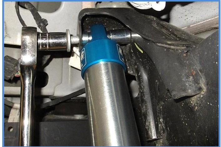
5. Place the rod end in the lower mount and install the factory bolt and nut. Tighten to factory specs.
