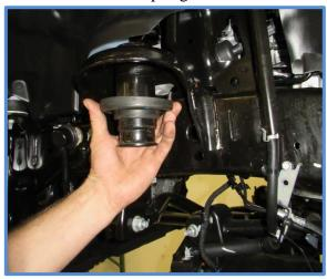
7. Mark 3" up from bottom of mount in a few spots and connect the dots making a nice line around the mount.
