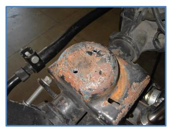
5. Install the 1/4" bolts provided in the kit to make sure the holes line up but don't install the nuts yet. Cycle the suspension again with the spacer in place and adjust bump stops to the desired position.
