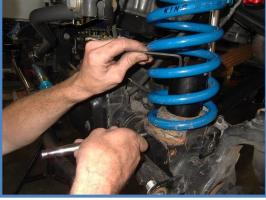
9. With the springs and spacers installed you can reinstall shocks, sway bar links, brake lines etc. as per the instructions starting with step 15 in the bump stop instructions.
