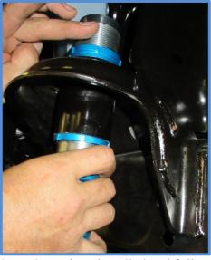
13. Now is the perfect time to set up your bump stops. Install your shocks without the springs installed and fully compress the suspension. Now adjust the bump stop so that it bottoms out just before the shock does. (See Bump Stop Memo and Cycling Suspension notes at the end of these instructions for more info.)
