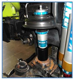
6. Once the bump stop position has been determined, tighten the locking nuts/collars and set screws.
