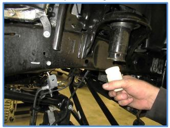
6. Remove the rubber spring isolator.
