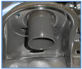
11. Once the cutting and trimming is complete you can mount the bump stop. Make sure the set screws are backed out before installing bump stop. Thread the bottom nut on all the way to the end of the threads.
