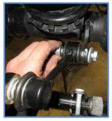
3. Unbolt the brake lines on both sides to get enough slack to push axle down when removing springs.
