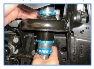
10. Prep the mount for install... do any final trimming/test fitting, then de-burr and paint the cut edge.
