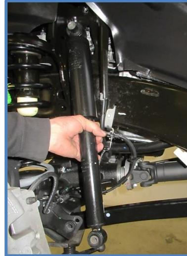
3. Install King Shocks using the factory hardware. Place the shock in the upper mount with the longer spacer facing in towards the frame. Insert the factory bolt and tighten to factory specs. Install shocks with cylinder on top and shaft mounted to the axle as shown.
