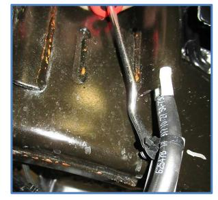
5. <u>Installing reservoir brackets</u> – First bolt the clamp to the reservoir bracket using the provided 1/4 X 1" FHCS (CB5501) using a 5/32 Allen wrench. Be aware the brackets are side specific. Photos show the RIGHT SIDE. See below for proper orientation.
