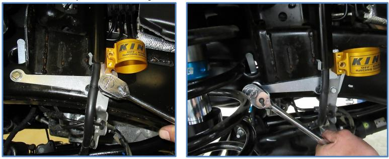
9. <u>Installing Shocks</u> – Be aware the shocks are side specific, make sure you have the proper shock for the side you are working on (photos below show LEFT SIDE). Begin placing the shock into position on the vehicle while inserting the reservoir into the clamp. Place the end cap into the upper mount, install the factory bolt and tighten to 60 ft-lbs.
