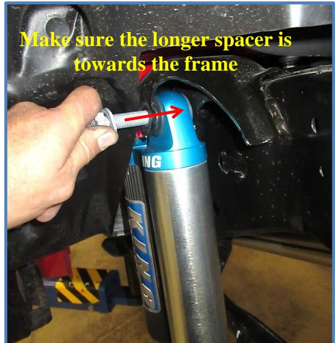
5. Place the rod end in the lower mount, install the factory hardware and tighten to factory specs.
