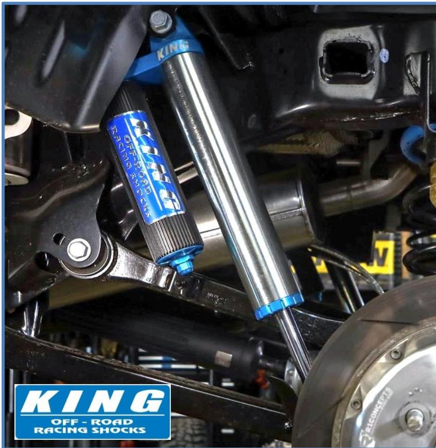
**DOUBLE CHECK ALL HARDWARE:** Make sure everything is installed correctly and all hardware is tight before reinstalling tires. Install tires, remove jack stands and lower vehicle to the ground. Recheck all hardware and lug nuts after 100 miles and periodically after that as part of routine maintenance.
