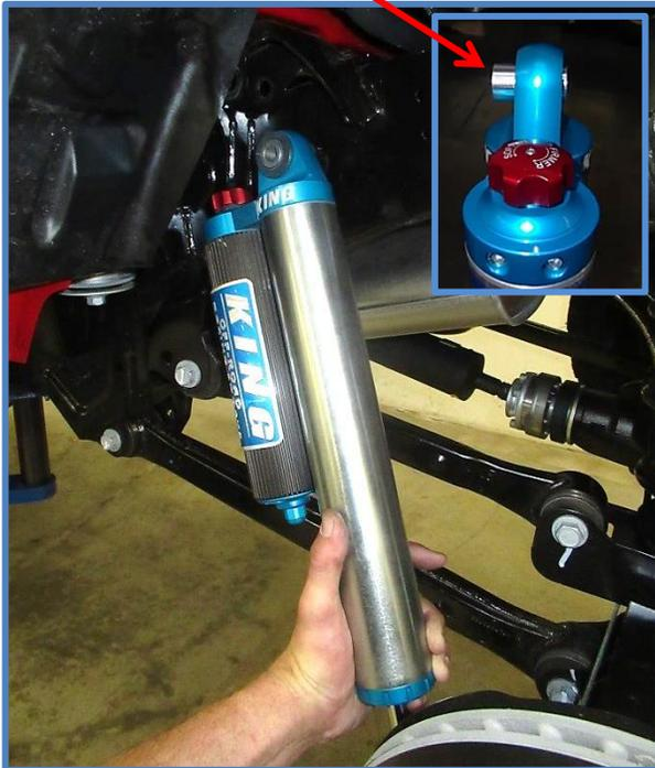
4. Place the factory bolt in the upper mount, install the nut and tighten to factory specs.
