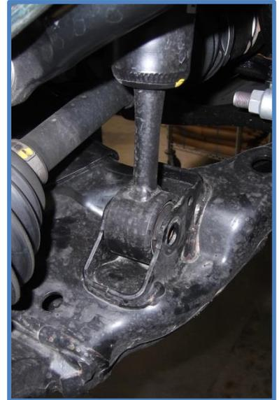
10. Remove the three nuts from the upper mount and remove shock.
