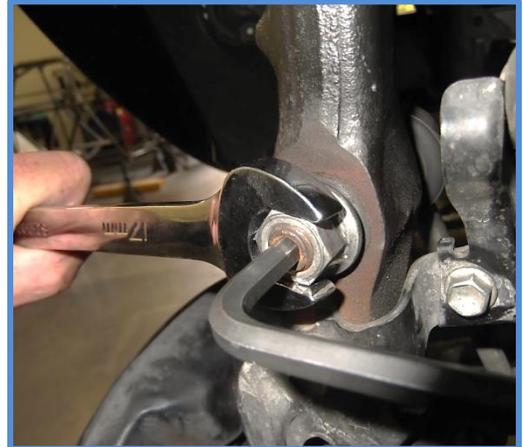
7. Pull the pin from the upper ball joint, loosen nut using a 19mm Socket and separate upper control arm from the steering knuckle.
