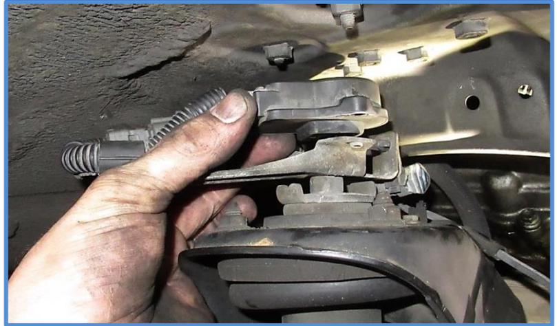
3. Remove bracket by holding nut on top of shock then remove the nut above the bracket.
