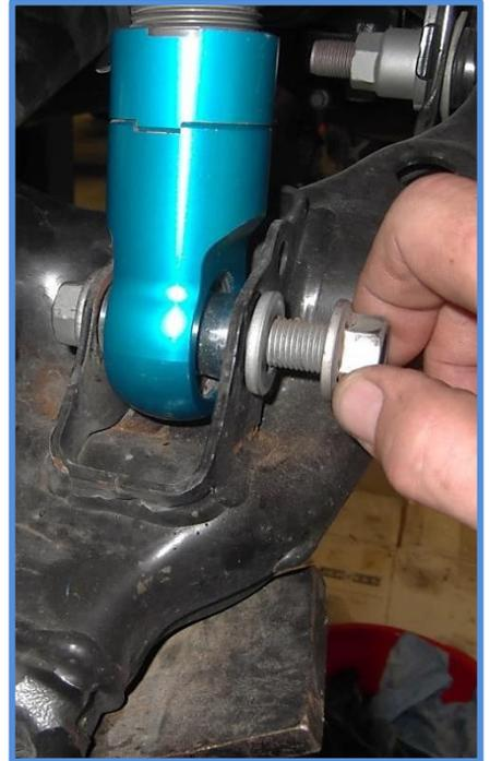
15. Jack up the lower control arm so the upper mounting plate is tight against the upper mount and install the 3/8 HD washers (CW1701) and 3/8 nuts (CN2711).
