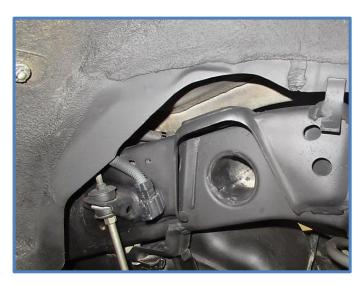
• You must also remove the factory bump stop and replace with a factory style 4Runner or FJ Cruiser bump stop. Failure to modify the bump stop will reduce available wheel travel and cause the rear axle to bottom out prematurely on the factory bump stops that were designed to work with the air bags.
