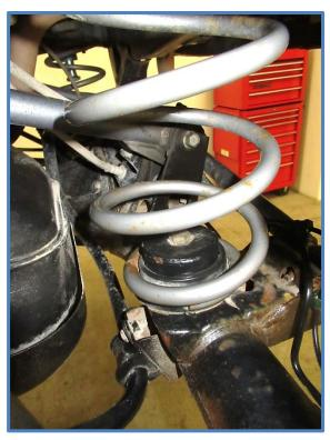
1. Assuming the coil swap has been performed - remove existing shocks (if applicable). Remove the lower mounting bolt from the stud mount on the axle. Remove nut from upper mount and remove shocks.
