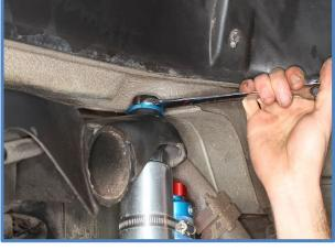
**Important Note:** The rubber bushings on your King Shocks are different from each other. Make sure the taller bushing is on the bottom next to the body of the shock as shown.
