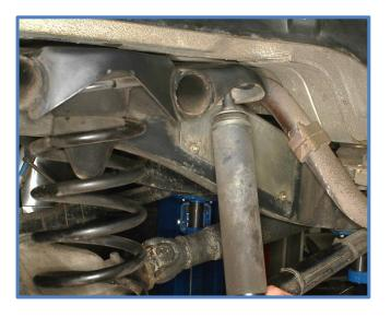
2. After removing stock shock, remove top plate and bushing and feed pin up into top mount. Place rubber bushing, blue plate, washer and nut on top mount but leave loose.
