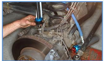
10. Only when the shaft is aligned with the hole, cut the strap on the shock so it extends. The shock is under pressure. Make sure your hands/fingers are clear of the extending shock. Install the sleeve, lower bushing, blue anodized plate, washer and the nut on the end of the shaft and tighten until the bushing starts to compress as shown \*Do not overtighten.
