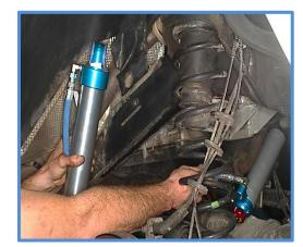
9. Remove the sleeve and lower rubber bushing from the end of the shaft and align shaft in hole on the lower mount.
