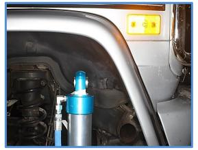
8. Bolt shock into upper mount as shown. Take care that the a/c line does not touch the shock. You might need to move it slightly.
