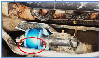
7. Before installing the shock, pass the reservoir and hose around behind the coil spring and brake lines as shown below.
