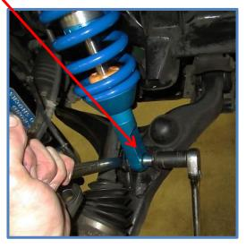
14. Once the shocks are in position and the upper bolts have been torqued you can replace the battery tray and battery and reassemble the air box and intake in the opposite order they were removed.
