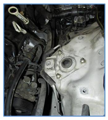
6. Remove air filter box on right side by first releasing the clips and unplugging the wiring from the sensor.
