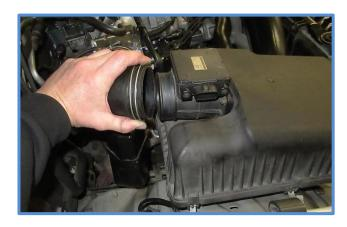
8. Remove cover and air filter to access bolts to remove air box.
