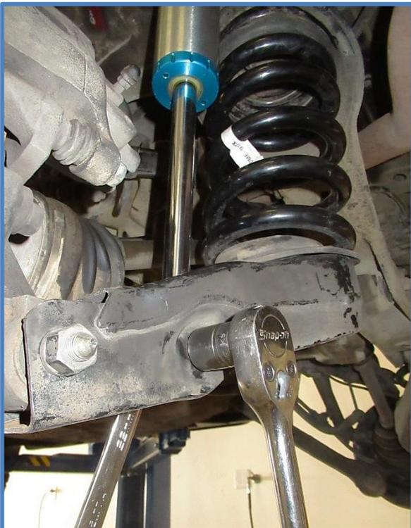
**Important Note:** The rubber bushings on your King shocks are different from each other. Make sure the taller bushing is on the bottom next to the body of the shock as shown. The silver washer between the rubber bushings represents the material thickness of the upper shock mount. It's important to tighten the nut only until the rubber bushings start to compress. There should be approximately 1/8" of the mounting pin protruding above the nut.
