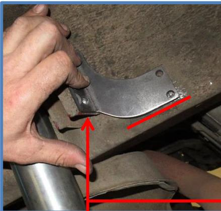
**Hold bracket against the body as shown, line up the bottom edge of flange on bracket with bottom edge of shock mount.**
