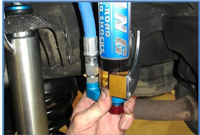
7. Attach bracket to vehicle by inserting the supplied M8 bolts (CB3825) into the bracket, then swing the bracket around and insert the bolts into the previously drilled holes. Install the M8 washers, nuts and tighten.
