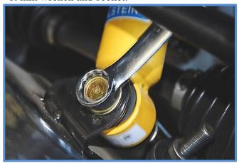
4. To gain more clearance to remove the old shock and to reinstall the new King Coilover shock you must unbolt the ABS bracket using a 12mm wrench or socket. Unbolt ABS bracket and remove the old shock.
