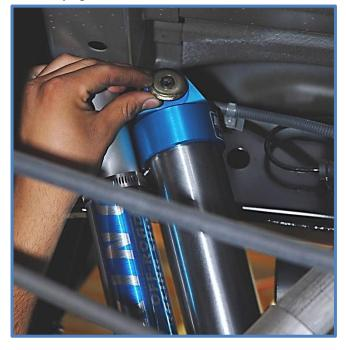
4. Reuse the factory bolt in the lower mount and tighten to factory specs using a 19mm socket and 19mm wrench. Make sure shocks are mounted so the reservoirs are facing away from axle.
