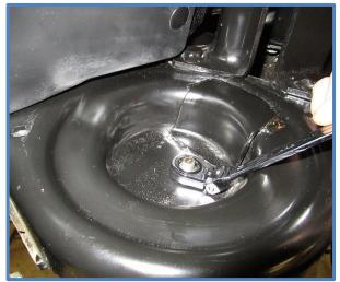
4. You are now ready to drill the hole in the coil bucket to accept the King bump stop. First you will need a 2-5/16 (2.3125") hole saw. Remove the pilot drill bit from the hole saw and install the hole saw adaptor provided in the kit as shown below.
