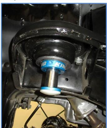
10. Cycling suspension and adjusting bump stops – Now that the bump stops are installed you will need to adjust the position so the bump stop is setup properly for your vehicle. With the coil springs removed and the shocks installed, jack the axle up until the shocks are bottomed out (Fully Compressed). Now adjust the bump stop so that it bottoms out just before the shock does.
