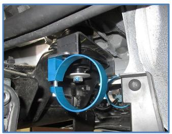
8. Slide the reservoir into the reservoir clamps, adjust position and install the 1/4 X 1" SHCS (CB1501). Tighten screws using a 3/16 Allen wrench.
