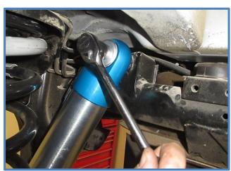
4. Place the spacer on the lower mounting stud followed by the rod end, then place the other spacer on the mounting stud and install the factory washer and nut. Tighten all hardware to factory specs.
