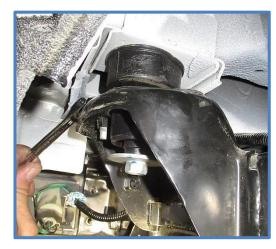
6. Attach the reservoir clamps to the reservoir bracket using the supplied hardware. Place the clamp on the bracket as shown below and install the provided 1/4 X 1/2" BHCS (CB2420). Use high strength thread lock on these screws to ensure the clamps stay secure.
