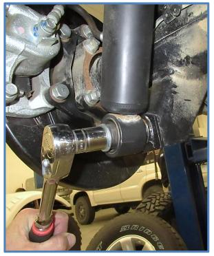
2. Remove the nut from the upper mounting stud using a 19mm wrench or socket and remove shocks.
